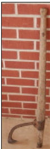
In the last issue, I asked you to identify this tool. The correct answer is a cant hook. A cant is a squared-off log at a saw mill. The first step in sawing a round log into lumber is to make it square by slicing off one side of the log, turning it over and repeating the cut on the other sides. What is left is called a “cant” which can then be cut into lumber. This tool was used to turn the log for the next cut. It can be used to turn any log for whatever reason.
