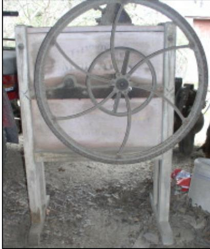
The correct answer to the “What Is It?” from last issue is a corn sheller. Some corn shellers are much smaller than this one. This one stands about four feet tall and is probably a deluxe model. It does an excellent job of shelling field corn after the husks are removed. The corn is fed into the chute at the top. When the handle is turned, the shelled corn will come out a chute at the bottom and the cob will be ejected.
